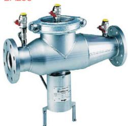
The BA298 is a backflow preventer suitable for protection against back pressure, backflow and back siphonage for fluids up to category 4. It is particularly suitable for industrial and commercial applications.
