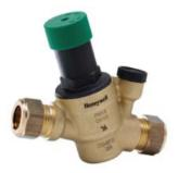
The D04FS is designed to protect household appliances against excessive supply pressures. A small compact valve that will maintain a constant water pressure irrespective of the supply pressure, which is often much higher.
