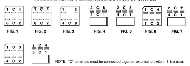
Refer to EECO Switch document "Soldering and Cleaning Specifications" for processing information.
